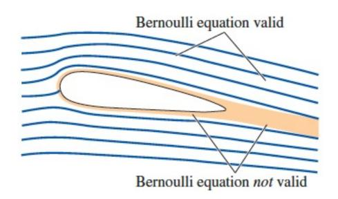
The sum of the kinetic, potential, and flow energies of a fluid particle is constant along a streamline, during steady flow, when compressibility and frictional effects are negligible.
