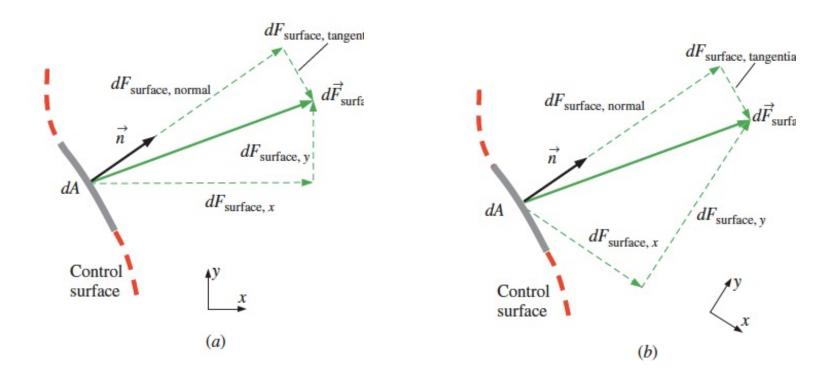
Surface force acting on a differential surface element:  $d\vec{F}_{\text{surface}} = \sigma_{ij} \cdot \vec{n} dA$
