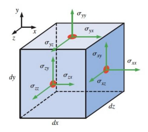
$\sigma_{ij}$  is the force per unit area in the direction of j through the plane (perpendicular to) i
