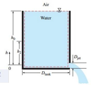
$$\int_{0}^{t} dt = -\frac{D_{\text{tank}}^{2}}{D_{\text{jet}}^{2} \sqrt{2g}} \int_{h_{0}}^{h_{2}} \frac{dh}{\sqrt{h}} \to t = \frac{\sqrt{h_{0}} - \sqrt{h_{2}}}{\sqrt{g/2}} \left(\frac{D_{\text{tank}}}{D_{\text{jet}}}\right)^{2}$$
