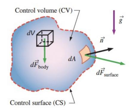
The forces acting on a control volume consist of body forces that act throughout the entire body of the control volume (such as gravity, electric, and magnetic forces) and surface forces that act on the control surface (such as pressure and viscous forces and reaction forces at points of contact).
